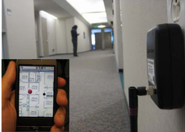
Figure 1. One of the wall-plugged nodes of the Cortina positioning system. On the left corner, a web page that displays the real-time position of the user.
