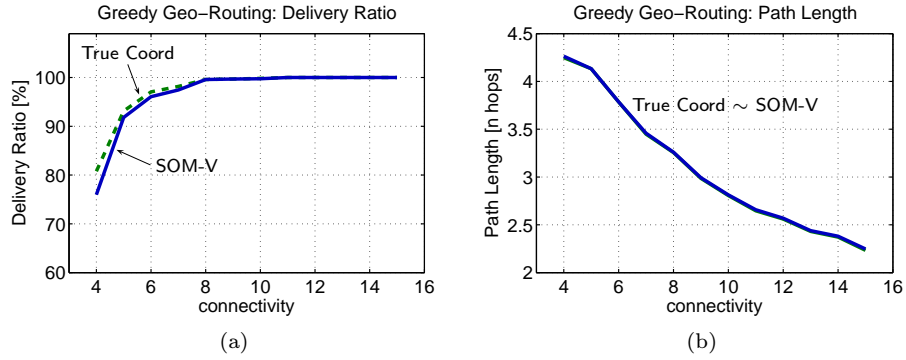
Fig. 8: Average performance of a greedy geo-routing algorithm using the true coordinates and the virtual maps produced by SOM-V. The path length plots (right) are almost completely overlapping for the two cases.
